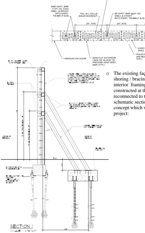
The existing façade framing will require shoring / bracing during the demolition of the interior framing and until the new framing in constructed at the second floor and roof and reconnected to the façade. Below is the schematic section showing the façade bracing concept which will be implemented in this project:
