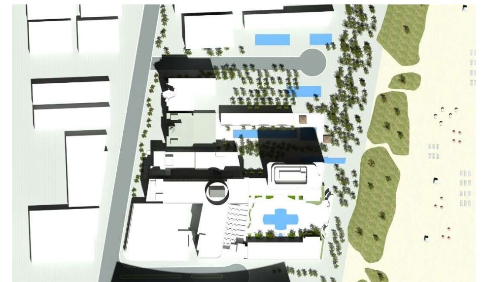
Figure 49. Shadowing at Equinox, noon, with proposed tower. (Heritage Architectural Associates with K4 Architecture)
