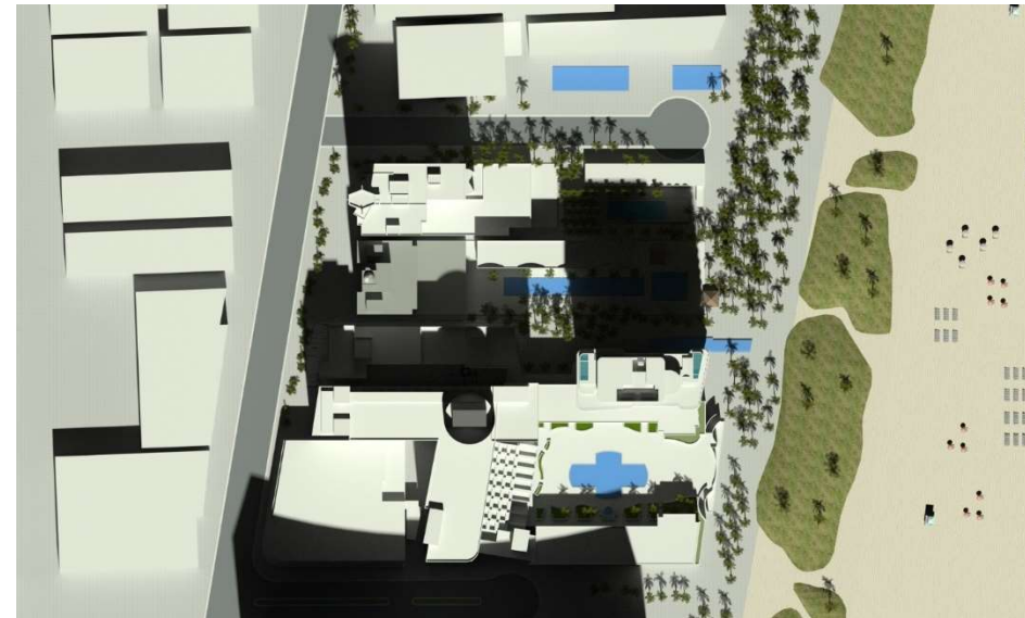
Figure 63. Shadowing at Winter Solstice, noon, with proposed tower. (Heritage Architectural Associates with K4 Architecture)
