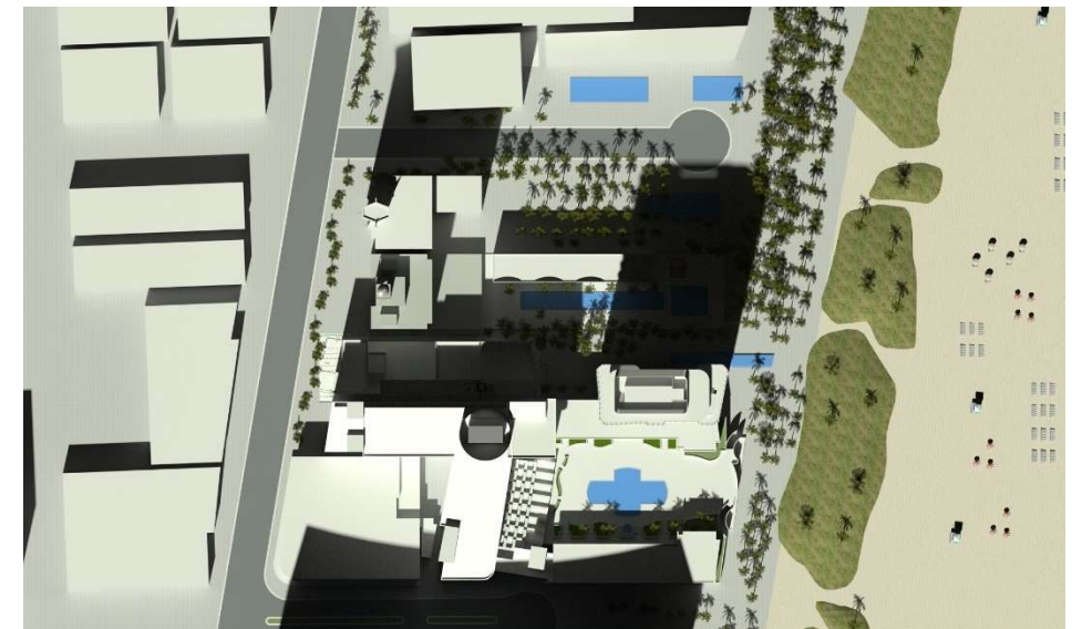
Figure 67. Shadowing at Winter Solstice, 1 p.m., with proposed tower. (Heritage Architectural Associates with K4 Architecture)
