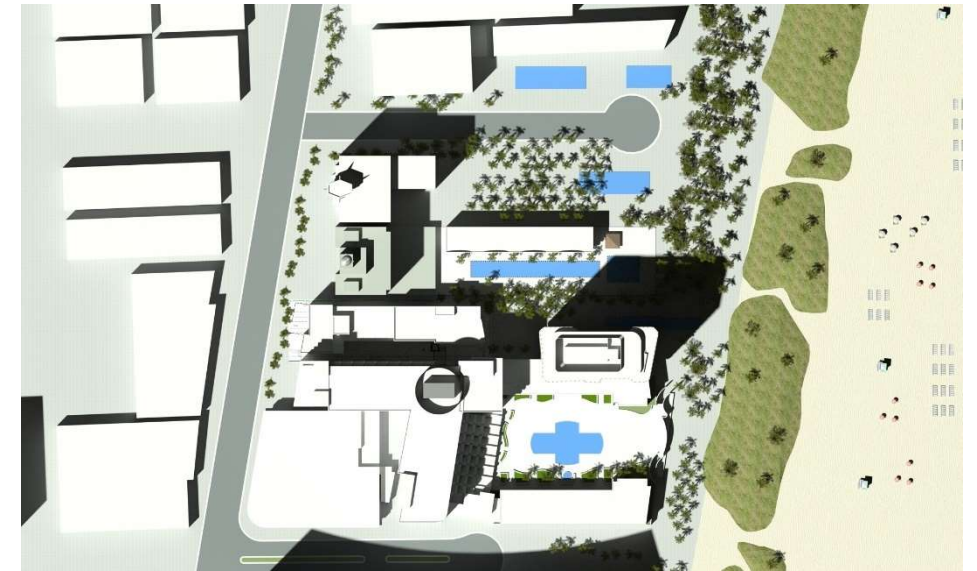
Figure 52. Shadowing at Equinox, 2 p.m., with proposed tower. (Heritage Architectural Associates with K4 Architecture)
