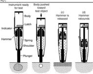
Fig. 2.2-Schematic to illustrate operation of the rebound
