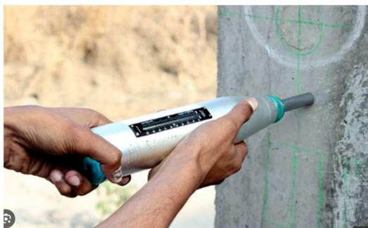
1. Hold the rod against the surface of concrete, press the instrument lightly, release the button, extend the rod when the pressure is relaxed hang the hook on the hammer.
