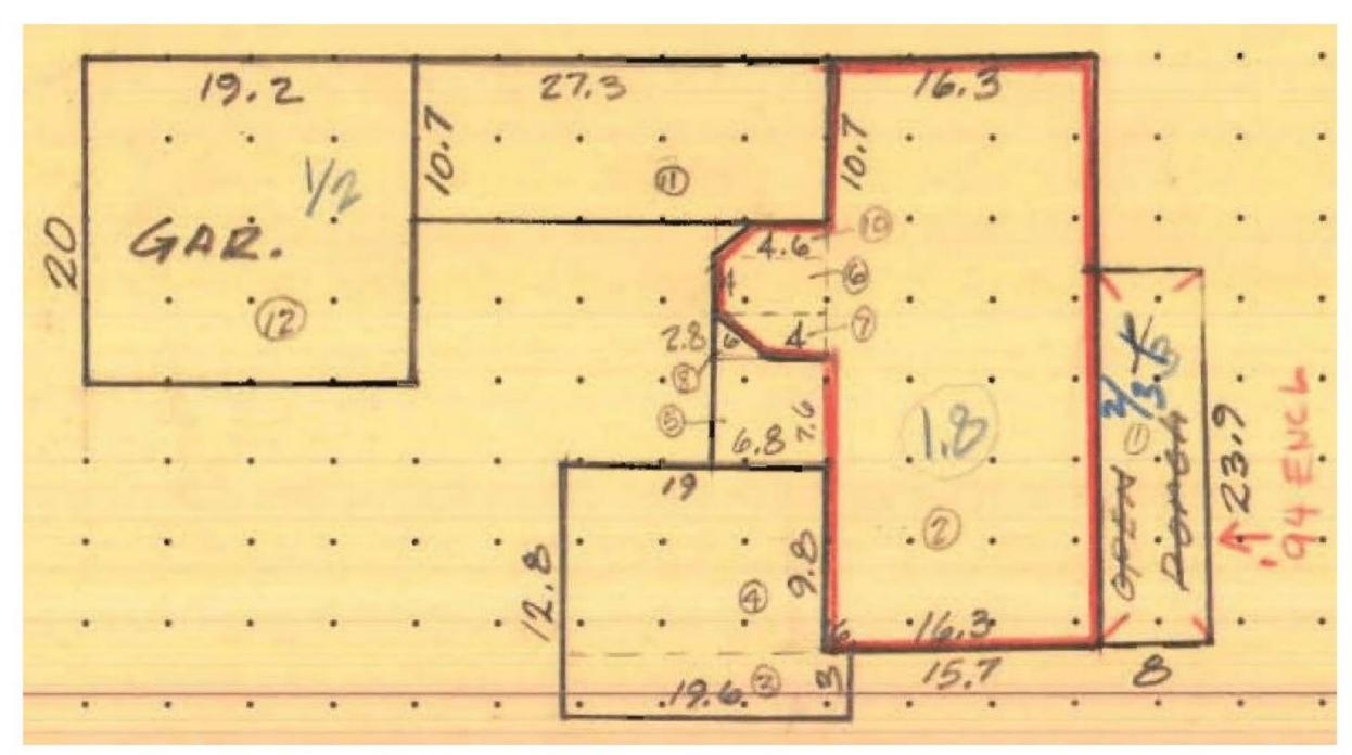
Figure 41 . Diagram of footprint of 7801 Atlantic Way indicating enclosure of east porch, 1994.
