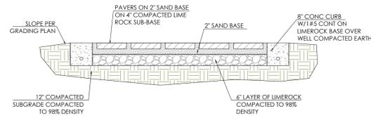
CONCRETE / BRICK PAVER DETAIL
