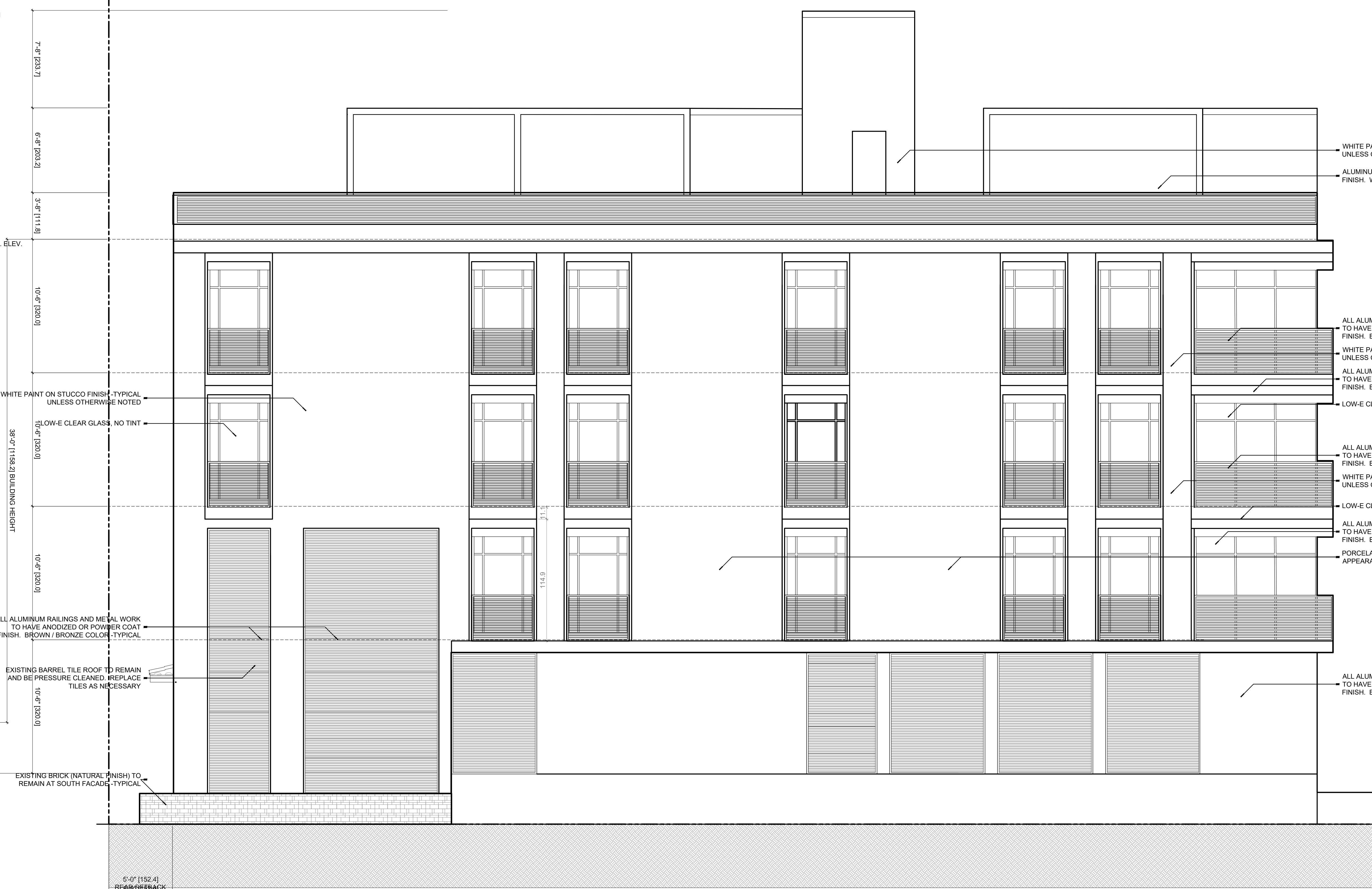
1 PROPOSED EAST ELEVATION @ ALLEY SCALE: 1/4" = 1'-0"
