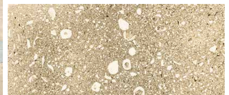
PROPOSED PRECAST CONCRETE PAVERS WITH EXPOSED SEASHELL FINISH
