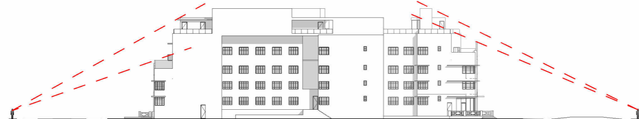
② SOUTH ELEVATION - LINE OF SIGHT - PROPOSED 1" = 60'-0"
