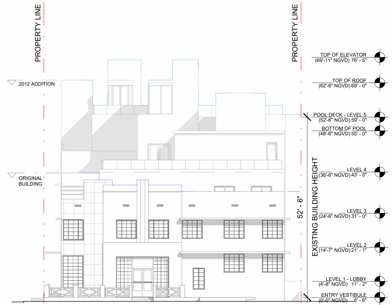
② WEST ELEVATION - EXISTING 1/16" = 1'-0"
