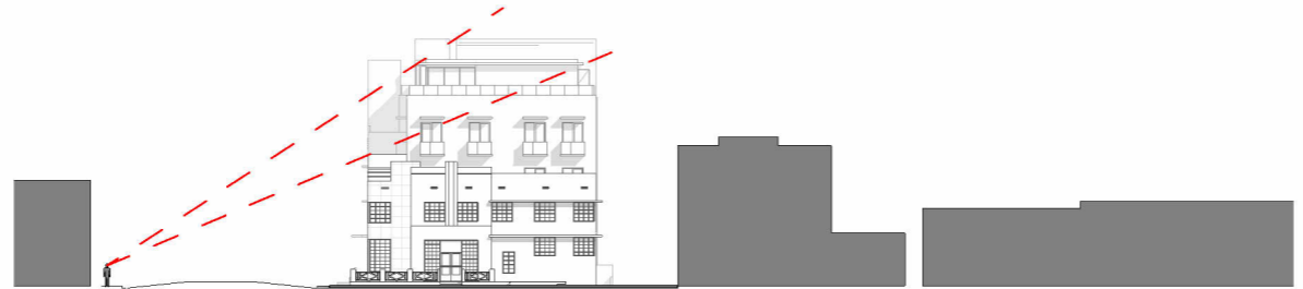
3 WEST ELEVATION - LINE OF SIGHT - PROPOSED 1" = 60'-0"
