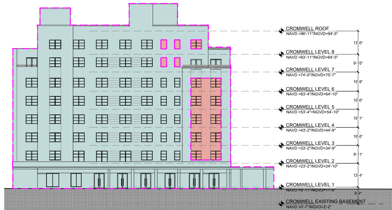
1 DEMOLITION CROMWELL SOUTH ELEVATION SCALE: 1/32" = 1'-0"
