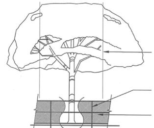
FENCE SHALL EXTEND A MINIMUM OF 8" BEYOND TRUNK FOR EVERY 1' OF DBH AS PER C.M.B. GUIDELINES.
