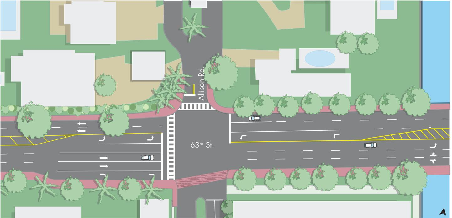
In this proposal a shared path is located on the south side of the bridge. Travel lanes have been narrowed to accommodate the needed bicycle pedestrian space.
