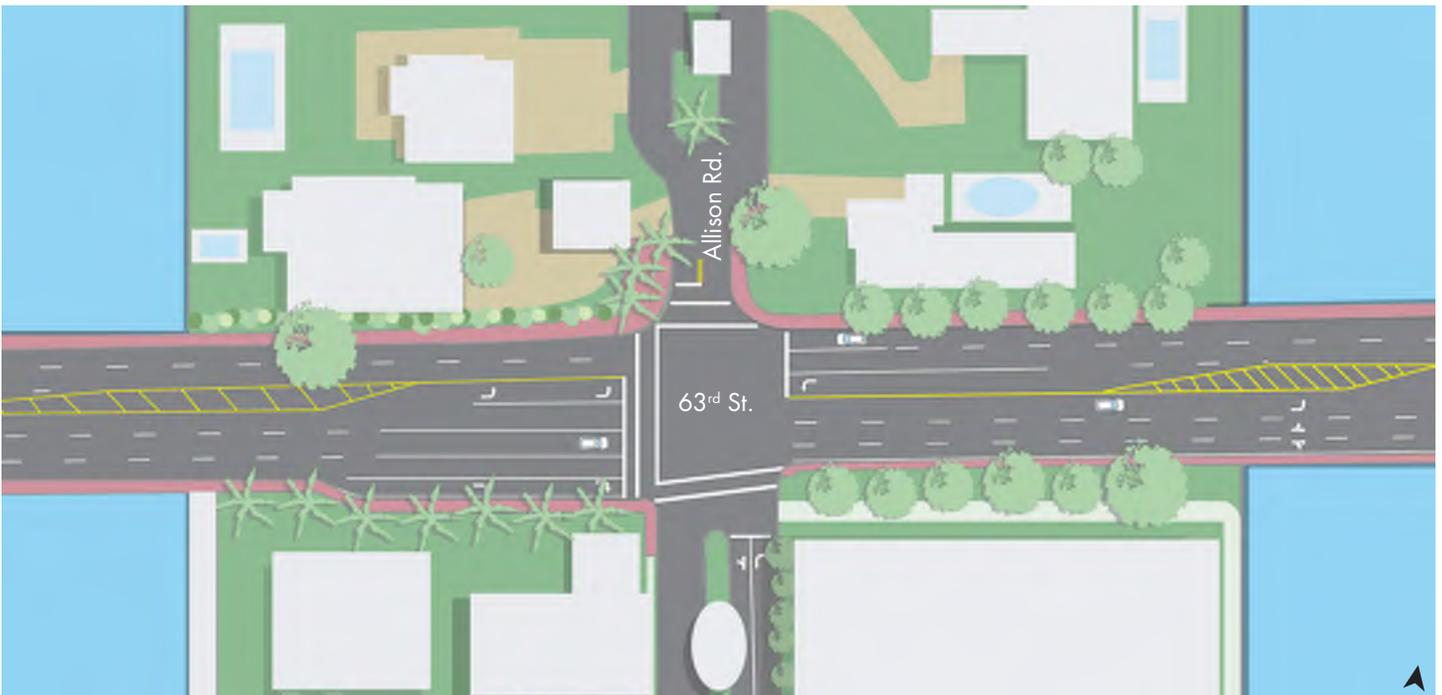
The proposal to add pedestrian and bicycle space to 63<sup>rd</sup> Street comes from the idea that this critical connection between the communities of Middle and North Beach needs a low-stress connection for the Type 3 riders. 63<sup>RD</sup> is a high speed, high volume corridor that requires a protected facility.
