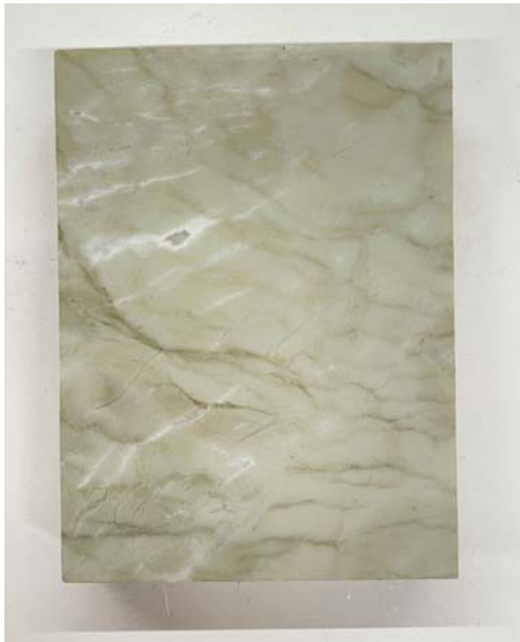
Honed green stone at fascia
