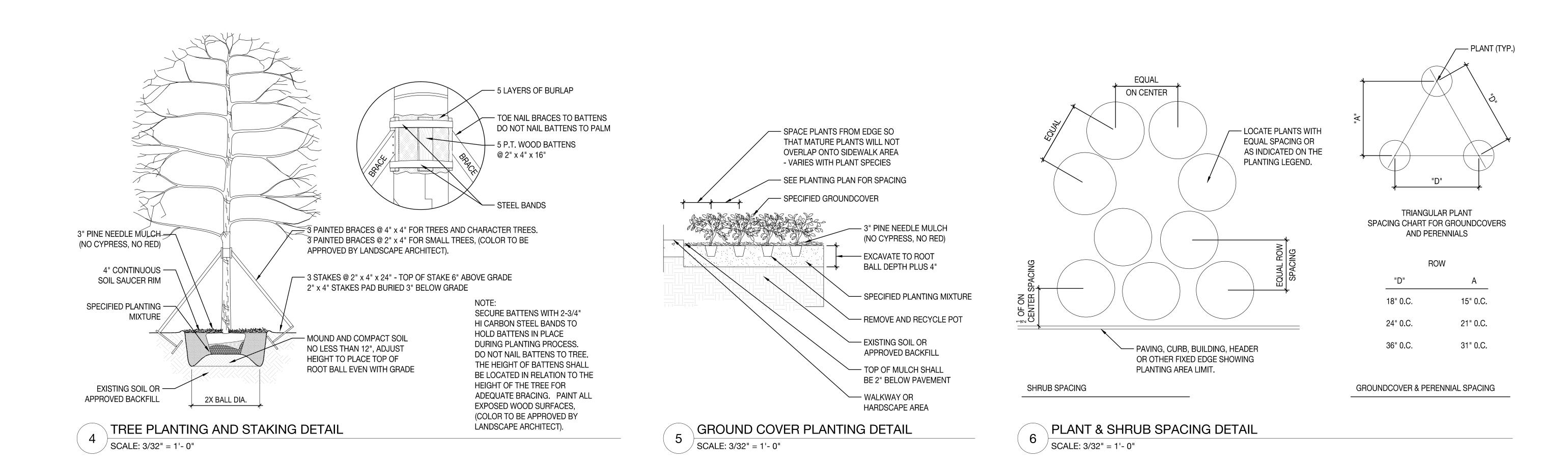
SECURE BATTENS WITH 2-3/4" HI CARBON STEEL BANDS TO HOLD BATTENS IN PLACE DURING PLANTING PROCESS. DO NOT NAIL BATTENS TO PALM. THE HEIGHT OF BATTENS SHALL BE LOCATED IN RELATION TO THE HEIGHT OF THE PALM FOR ADEQUATE BRACING. PAINT ALL EXPOSED WOOD SURFACES, (COLOR TO BE APPROVED BY LANDSCAPE ARCHITECT).
