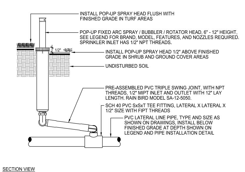
INSTALL SPRAY HEADS 4" FROM PAVING EDGE IN TURF AREAS. INSTALL SPRAY HEADS 6" FROM PAVING EDGE IN SHRUB AND GROUND COVER AREAS. INSTALL SPRAY HEADS 12" FROM THE FACE OF BUILDING WALLS OR WINDOWS. INSTALL SPRAY HEADS PLUMB. ADJUST NOZZLE SPRAY TO COVER THE LANDSCAPE AREA WITHOUT OVERSPRAY ONTO PAVING, FENCES, WALLS OR BUILDINGS. SPRINKLER, SWING JOINT, AND PVC FITTINGS SHALL ALL HAVE "NPT" STYLE THREADS
