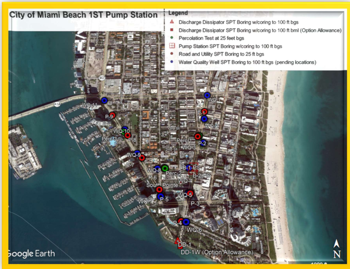
Figure 3: Preliminary Boring Location Plan as Provided by Jacobs Engineering to be Confirmed During Design Phase
