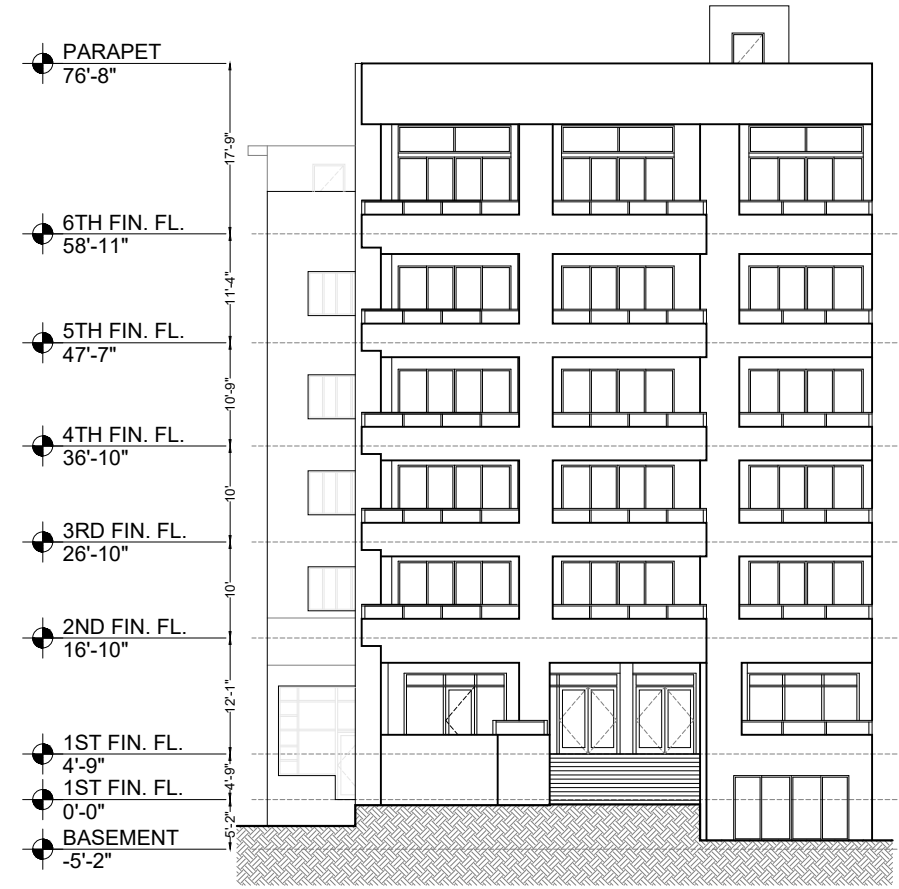
1 EXISTING EAST ELEVATION SCALE: 1" = 20'-0"
