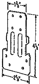
Figure 8a—RSP4 Stud Plate Connector Dimensions
