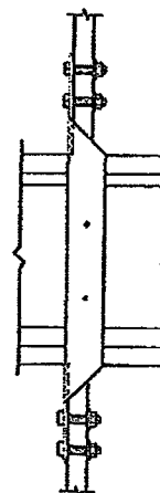
FIGURE 6b—FTA FLOOR TIE ANCHOR INSTALLATION (See Table 6)
