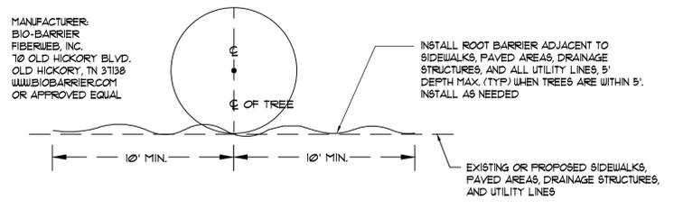
**5** ROOT BARRIER INSTALLATION SECTION NTS
