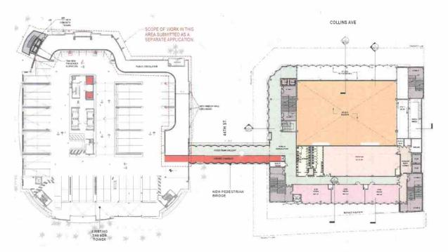
Proposed connection plan: 4<sup>th</sup> level Tresor Tower parking garage to 3<sup>rd</sup> level ballroom structure
