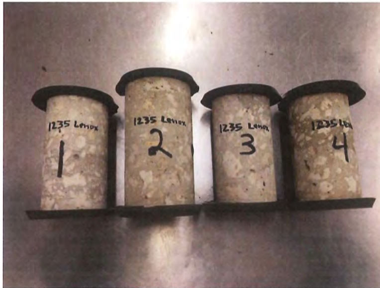
Figure 10: Photograph of Core Samples (Compressive Strength Tests)
