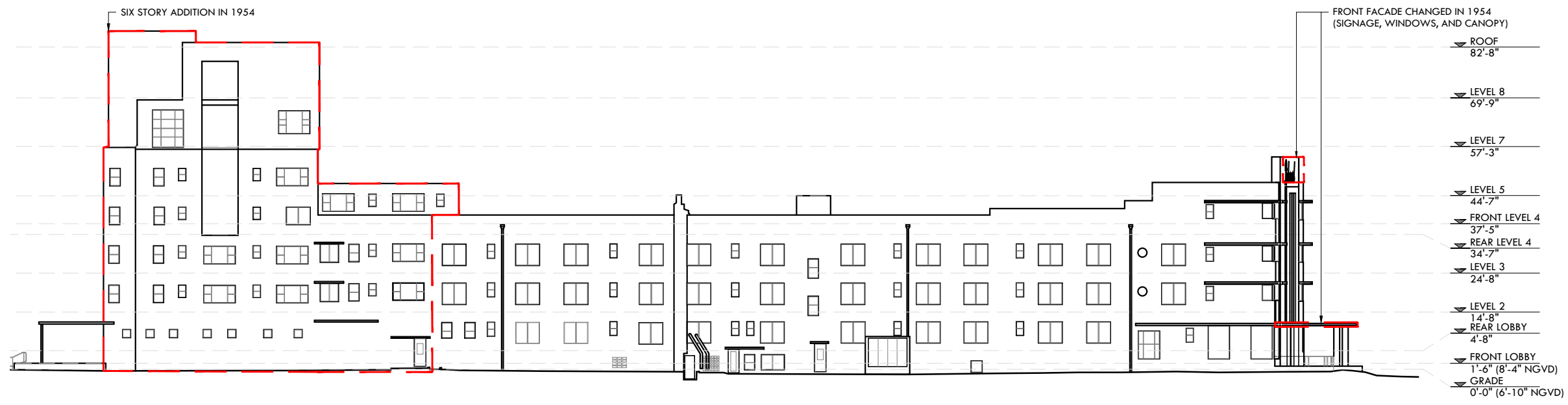
1 EXISTING ELEVATION - NORTH SCALE: 1/32" = 1'-0"
