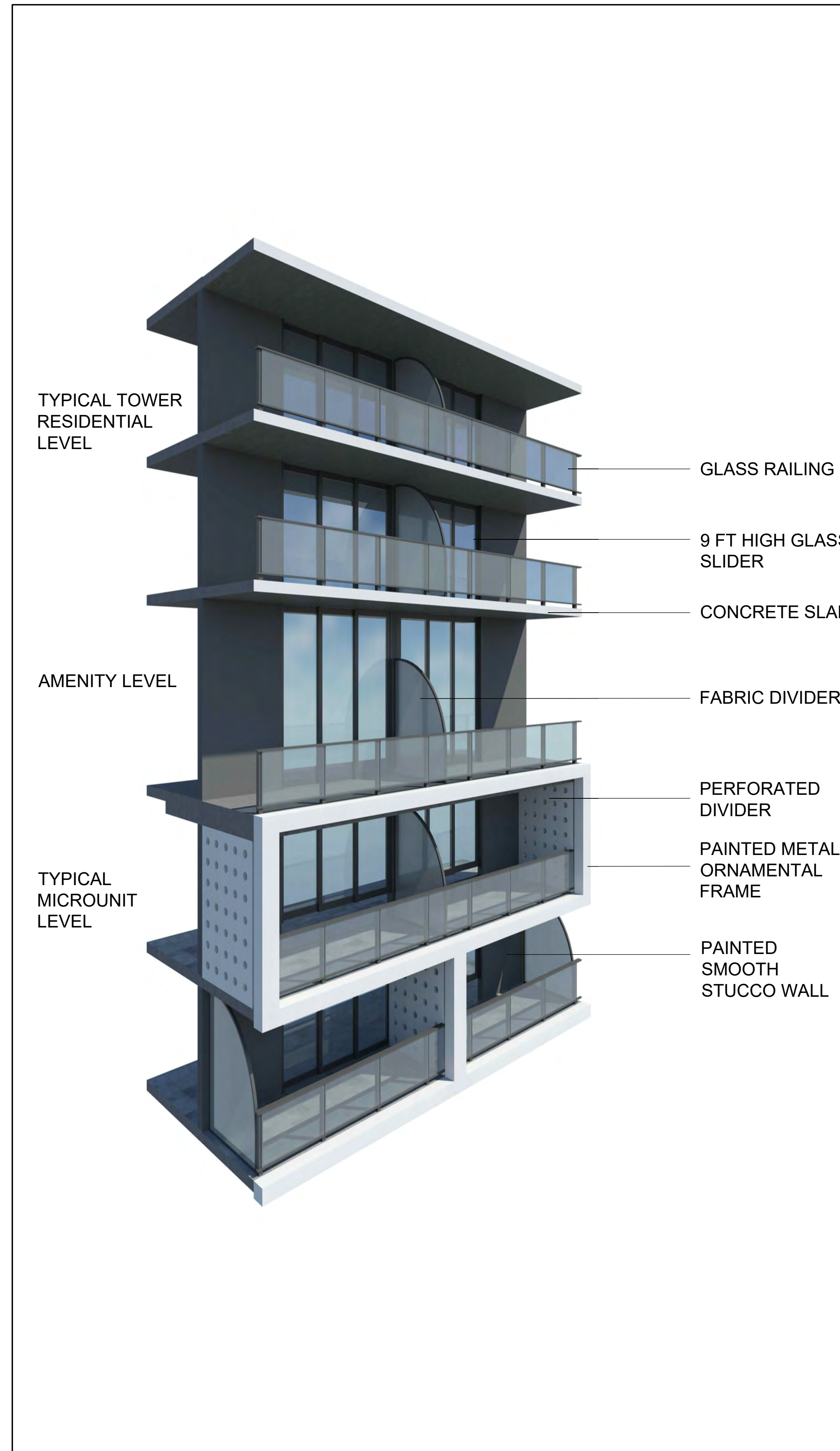
TYPICAL PODIUM LEVEL - AMENITY LEVEL FACADE
