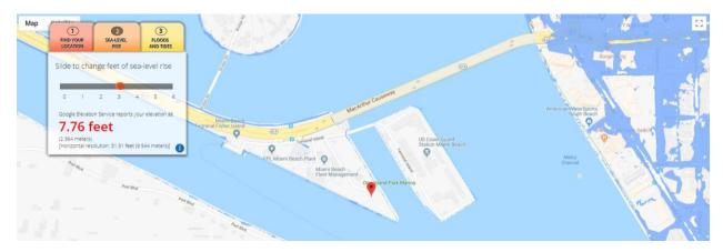
Figure 3 – Site Elevation 7.76-Feet with Sea Level Rise of 34-Inches at Year 2060
