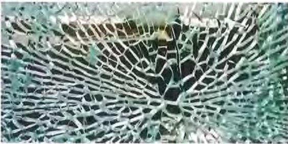
An example of tempered glass in its correct break pattern
