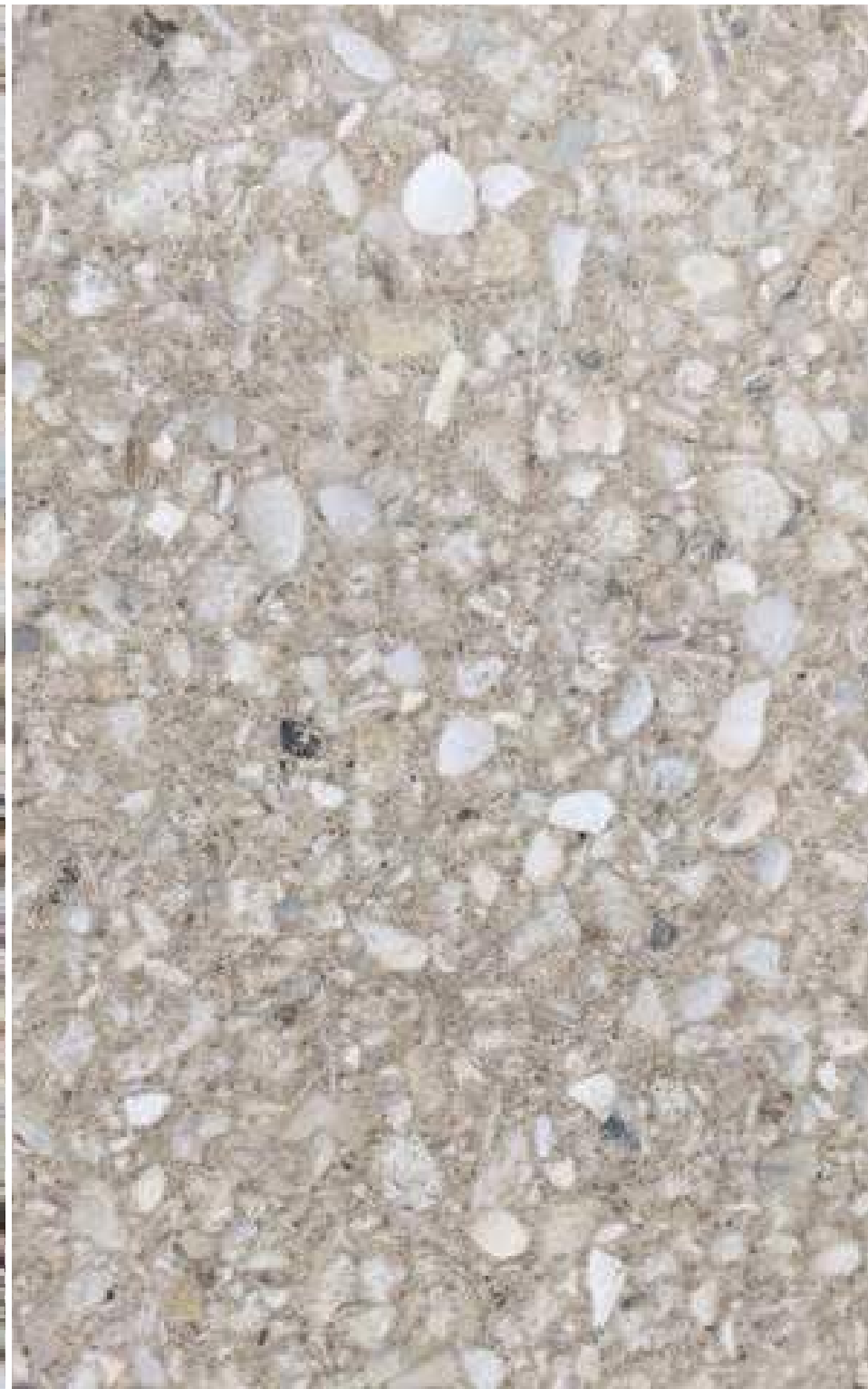
PV-101 Concrete with Shell
