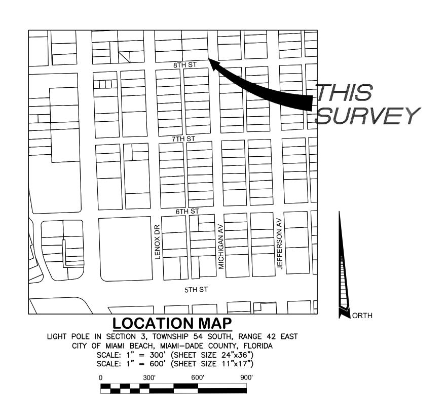
1. This is a Specific Purpose Radial Survey for the stated purpose of locating improvements within a 50' wide radius of the existing light pole to be used for proposed telecommunications equipment. Client provided the location of the subject
