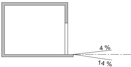
These illustrated maximum approach angles must **NOT** be exceeded. Incorrect approach angles will cause **SERIOUS MANEOUVRING & POSITIONING PROBLEMS** on the parking system for which the local agency of Klaus accepts no responsibility.
