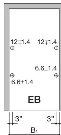
Units are bolted to the floor. Drilling depth approx. 6"
