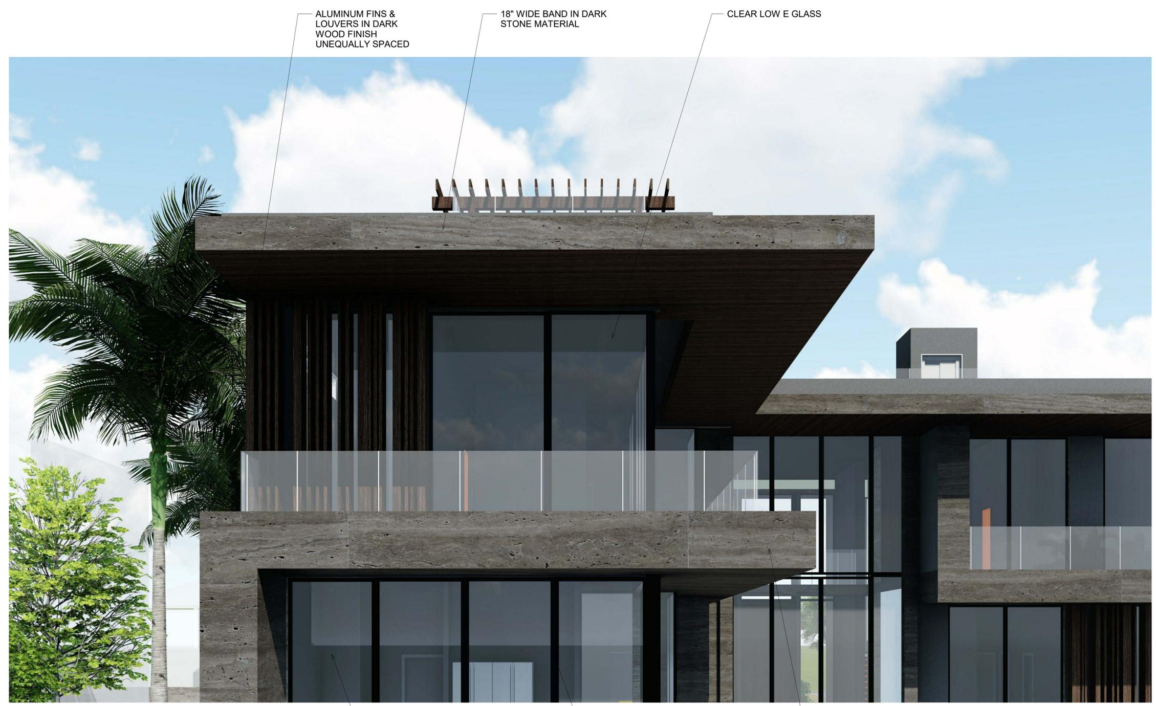
ALUMINUM FINNS & LOUVERS IN DARK WOOD FINISH UNEQUALLY SPACED
