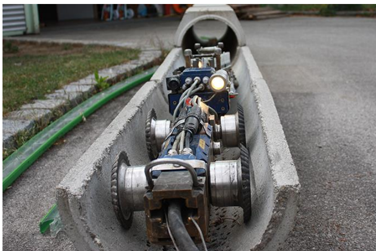
Figure 2-3: Current version of CableRunner robot used for installation of fiber optics in inaccessible sewers.
