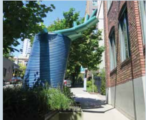
The ten-foot-high Beckoning Cistern distributes water down the hill in a series of cascading planters when it becomes full.
