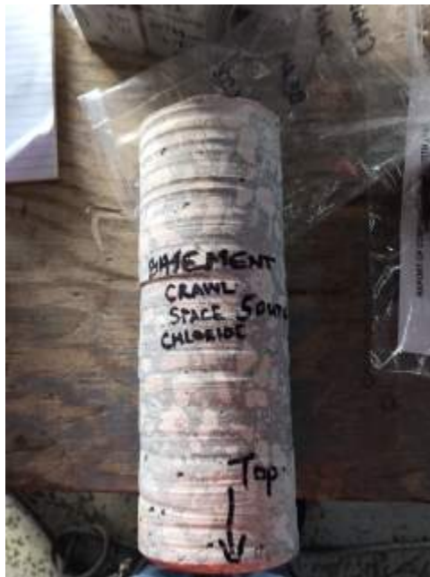
Figure 14: Core Sample – Chloride Test
