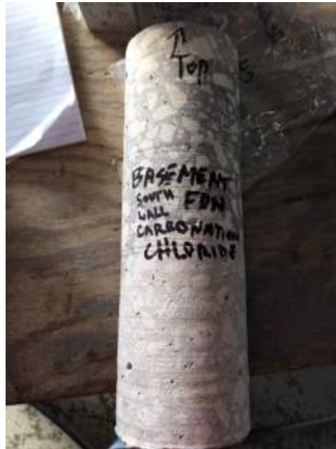
Figure 15: Core Sample – Chloride and Carbonation Tests
