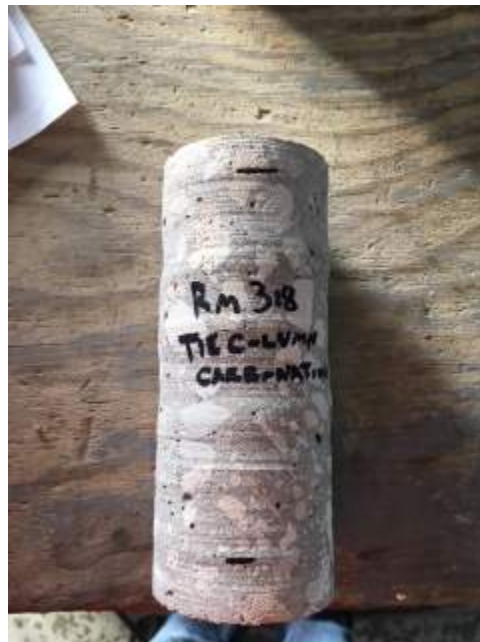
Figure 16: Core Sample – Carbonation Test
