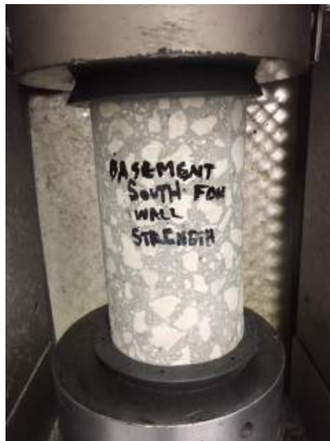
Figure 8: Core Sample – Compressive Strength Test
