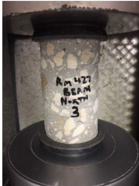
Figure 3: Core Sample – Compressive Strength Test
