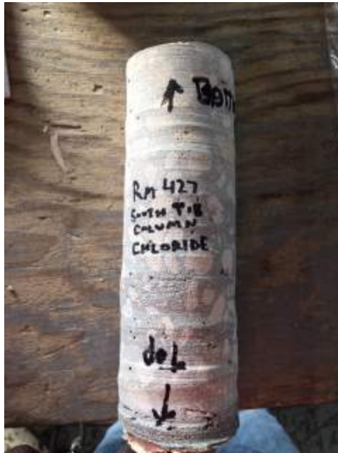
Figure 13: Core Sample – Chloride Test
