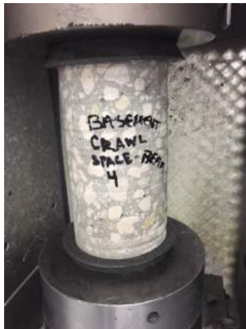
Figure 4: Core Sample – Compressive Strength Test
