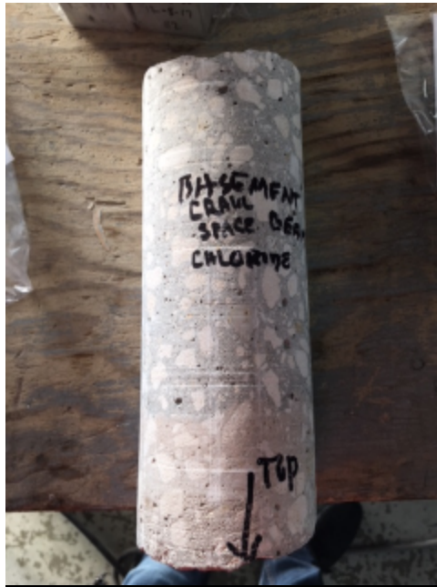
Figure 17: Core Sample – Chloride Test
