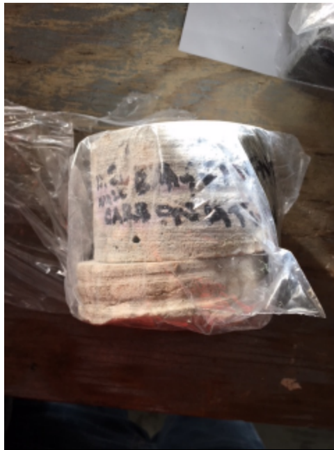
Figure 18: Core Sample – Carbonation Test
