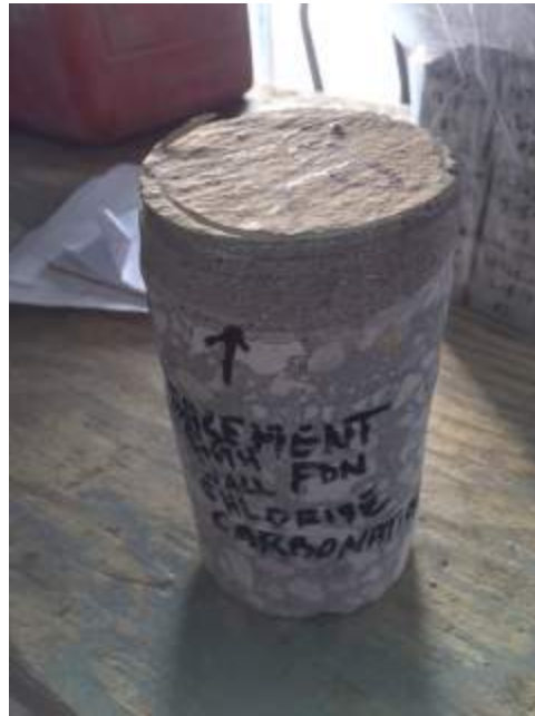
Figure 11: Core Sample – Chloride and Carbonation Tests
