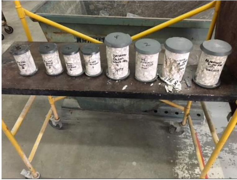
Figure 9: Core Samples – Trimmed/Capped/Tested
