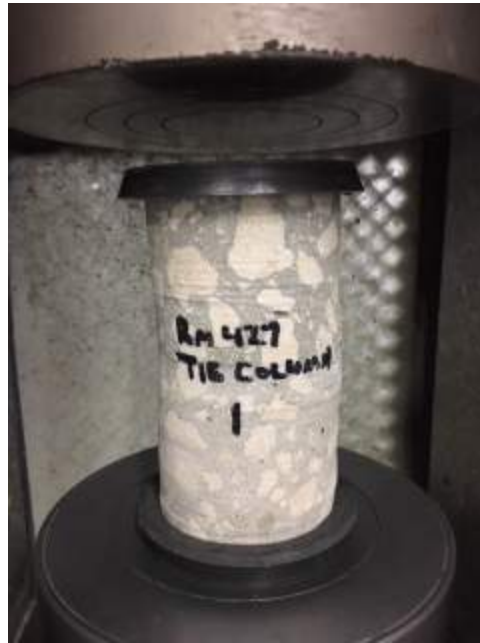
Figure 1: Core Sample – Compressive Strength Test
