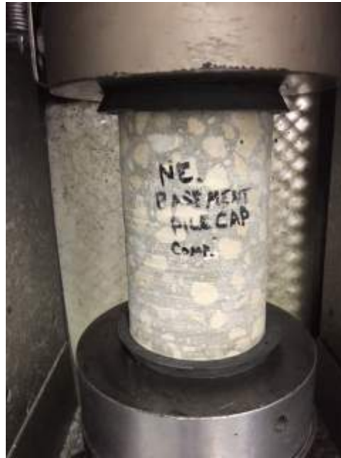
Figure 7: Core Sample – Compressive Strength Test
