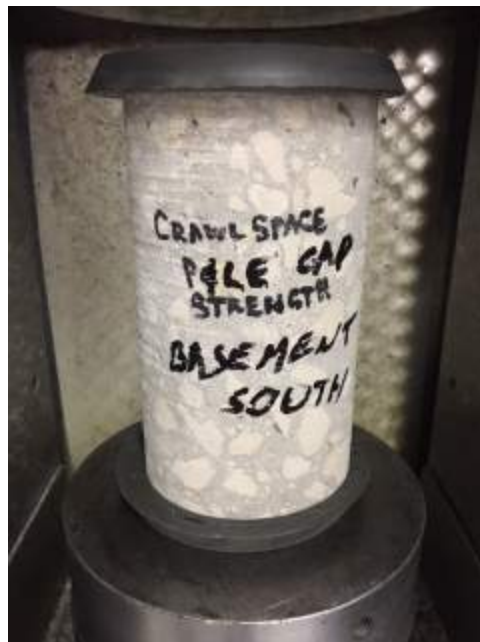
Figure 6: Core Sample – Compressive Strength Test
