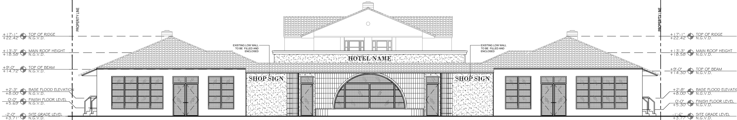
2A PROPOSED WEST ELEVATION SCHEME A SCALE : 3/32" = 1'-0"
