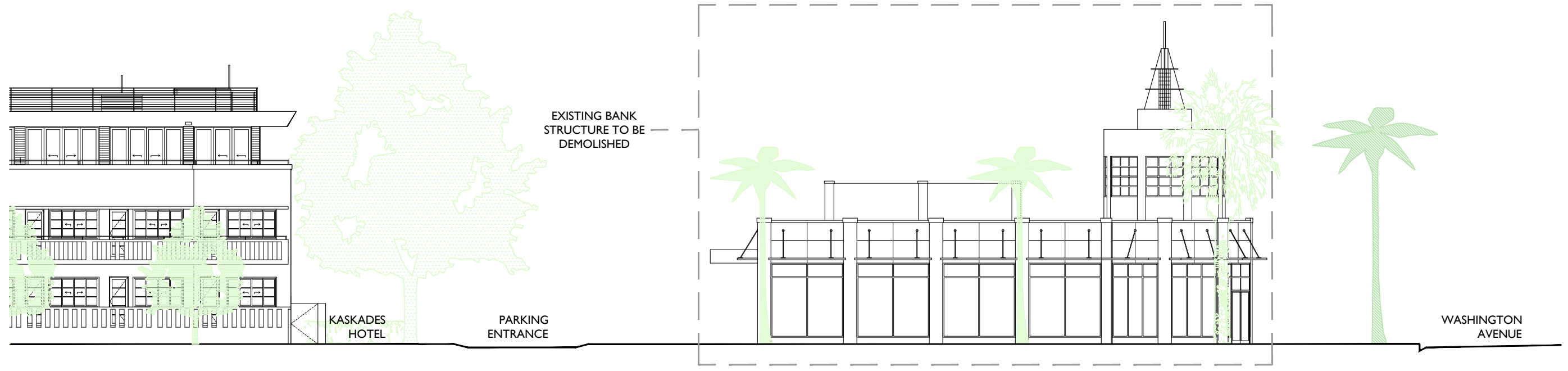
EXISTING NORTH ELEVATIONS SHOWING DEMOLITION 1/16" = 1'-0"
