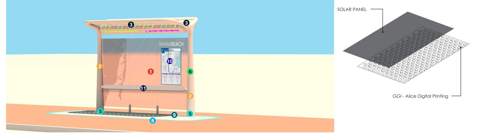
**1** GLASS - Optional Color gradient 3/8" thick, clear tempered glass with mylar film laminated between sheets to block UV rays.
