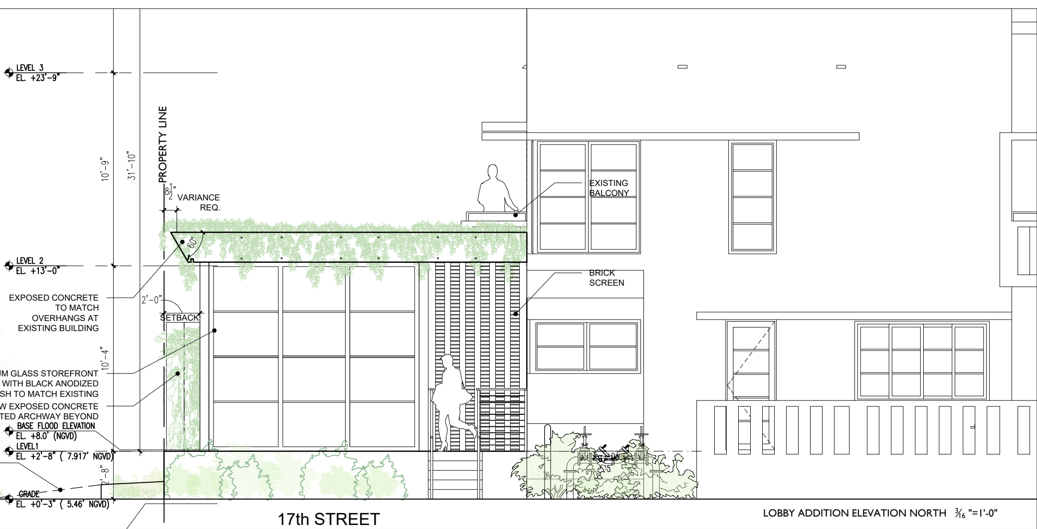
ALUMINUM GLASS STOREFRONT WITH BLACK ANODIZED FINISH TO MATCH EXISTING
