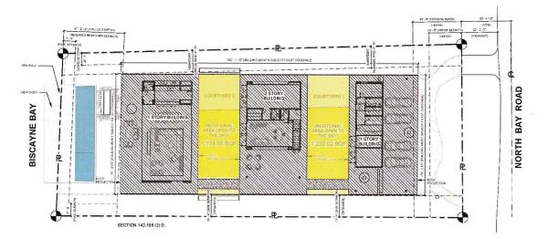
Further analysis of the lot coverage calculation also takes into account outdoor covered areas that are open on at least two sides. The Code exempts those covered areas that area attached to main building and project 10 feet or less from being included in the overall lot coverage calculations The areas highlighted below illustrate the nearly 3,520 SF of covered open areas that, in addition to uncovered outdoor area, constitute the excessive lot coverage of 53%.
