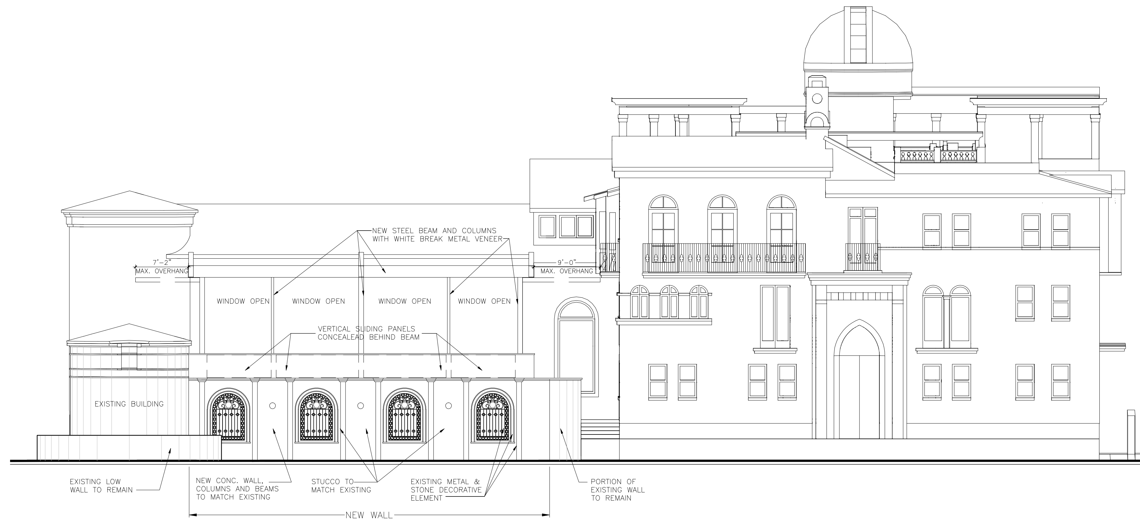
1 PROPOSED EXTERIOR FRONT ELEVATION (OPTION 1) - OPEN WINDOWS SCALE: 1/8" = 1'-0"
