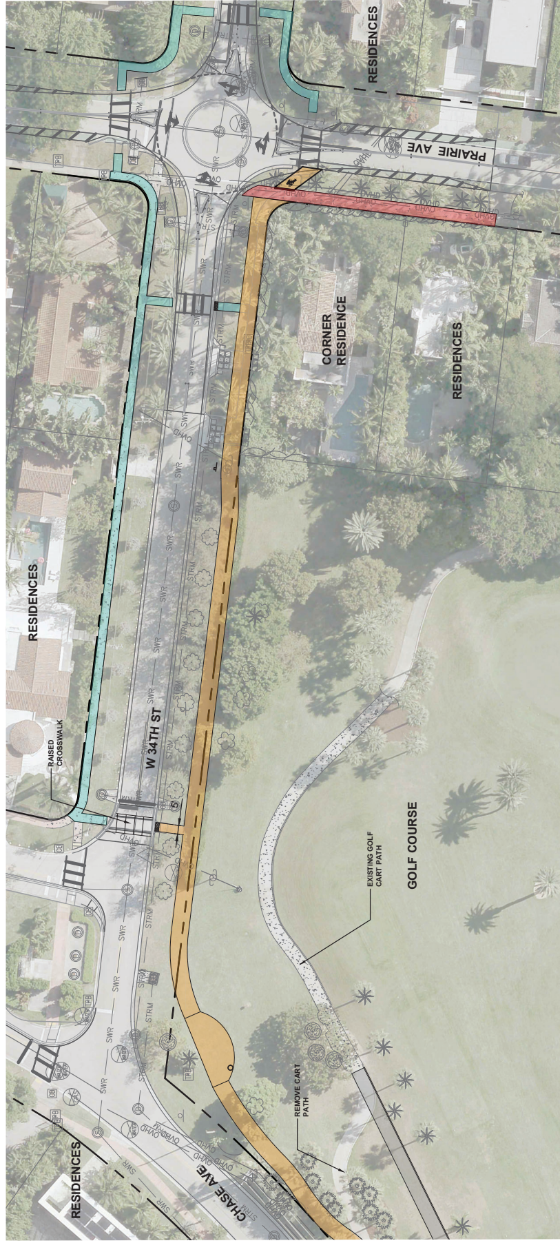
OPTION 1 : CURRENT DESIGN-10'-0" WIDE SHARED USE PATH ALONG W. 34TH STREET FROM CHASE AVENUE TO CONNECT WITH EXISTING SIDEWALK AND GREEN BIKE LANES ON PRAIRIE AVENUE.
