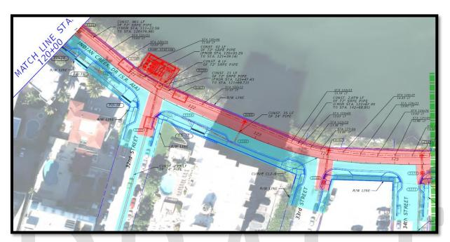
Phase 3: Construction of remaining 72" Trunk line from 32<sup>nd</sup> to 41<sup>st</sup> Street, Construction of side-street drainage system and Roadway Reconstruction (ITB Contract)
