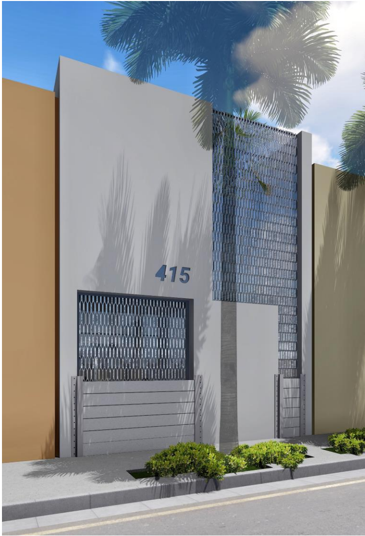
Closed Gate + DRY FLOODPROOFING Panel
