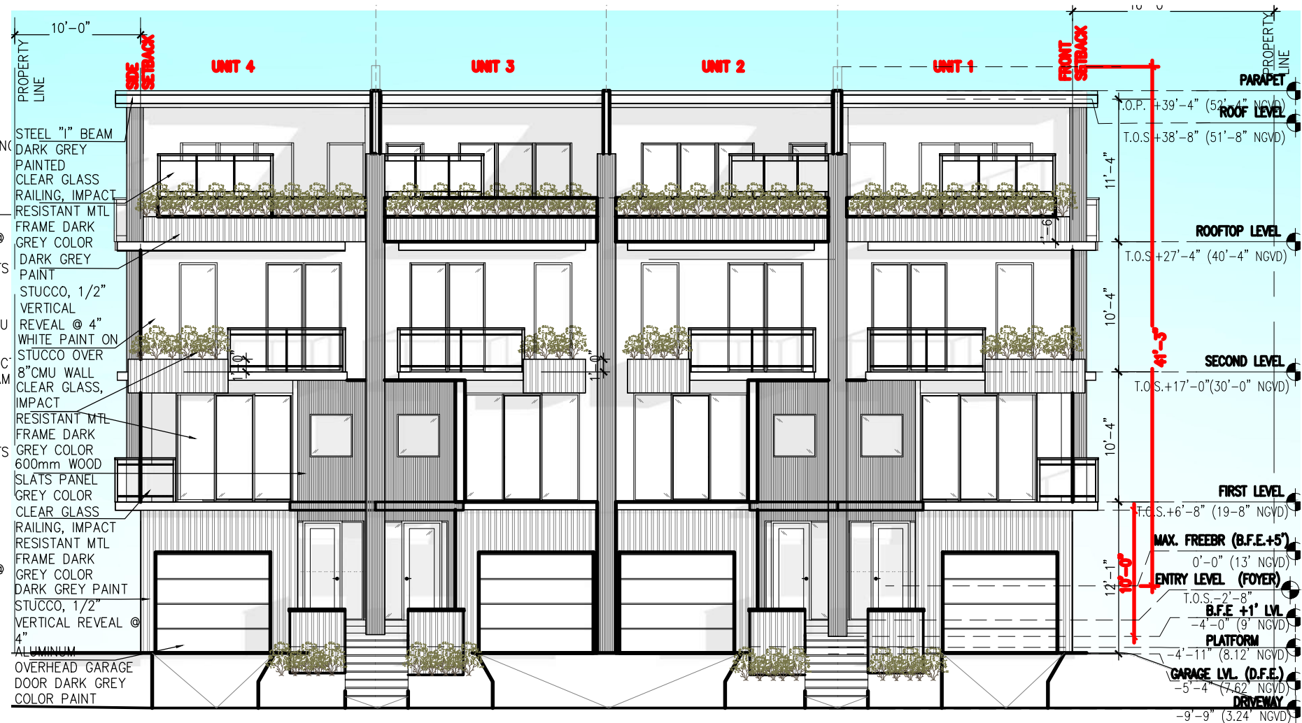
2 WEST ELEVATION SCALE: 3/32" = 1'-0"
