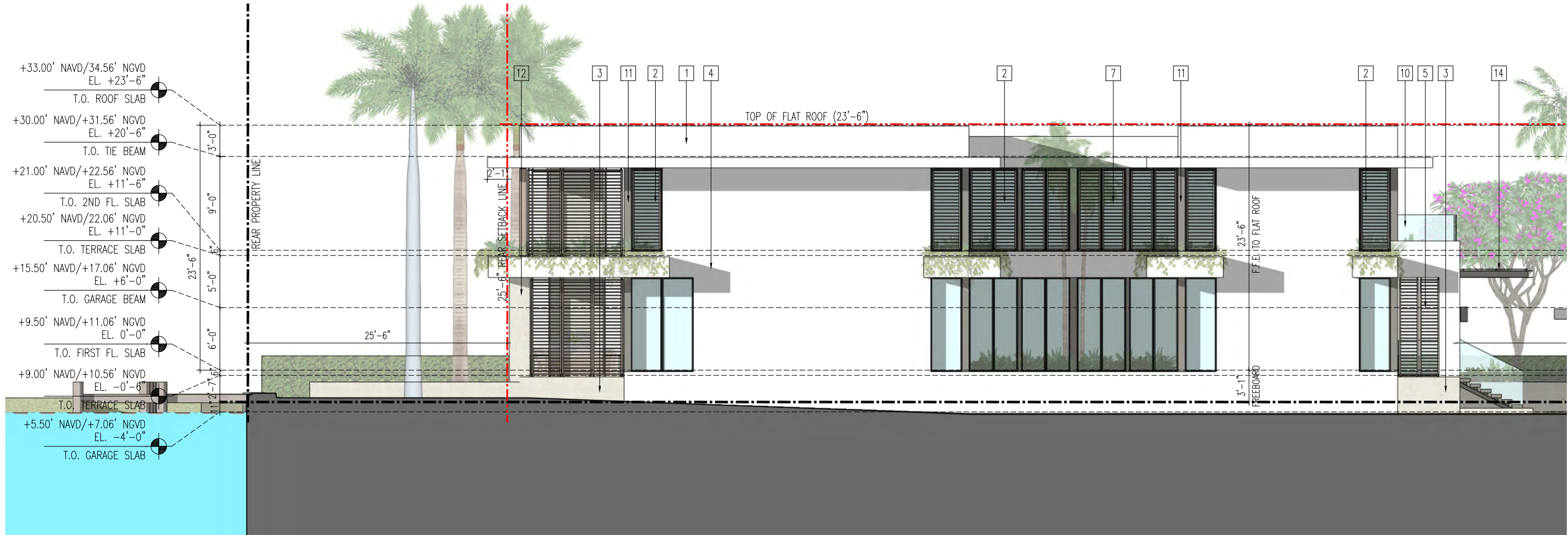
1 LOT 10 - EAST ELEVATION (PARTIAL) A1.0 | A5.3 3/32" = 1'-0"
