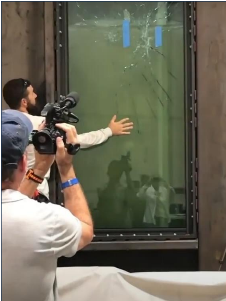
Figure 2. A flood glazing system is undergoing shop testing. The glass has been intentionally damaged to simulate potential wind-driven impacts coinciding with flood events. 3 This system may be a viable alternative for the historic atrium.
