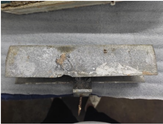
Detail of aluminum edge before mechanical and wet cleaning test.
