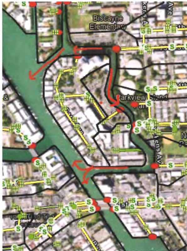
Figure V.7: Schematic of conceptualized tidal flushing during ebb tide, with more tidal flushing towards the south of Parkview Island. It is possible that tidal flushing through the PVC North is limited by the sharp 45-degree angles created by Biscayne Point Island and flows from the waterways to the north. In contrast, water exiting the PVC South could flow to the main waterway with less impedances.
