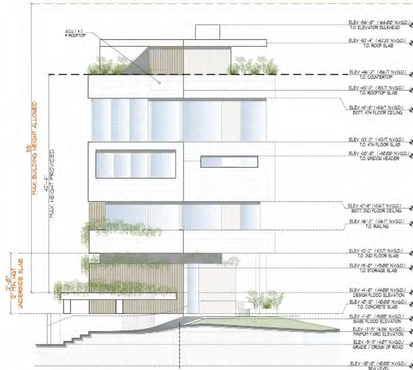
2 SOUTHEAST ELEVATION A3.1
