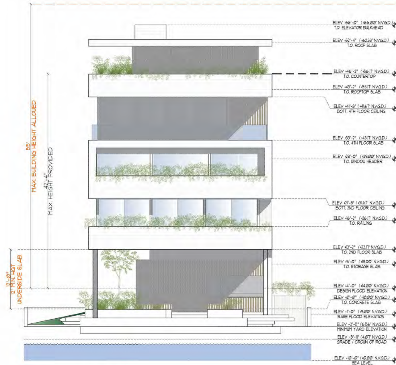
4 NORTHWEST ELEVATION A3.1
