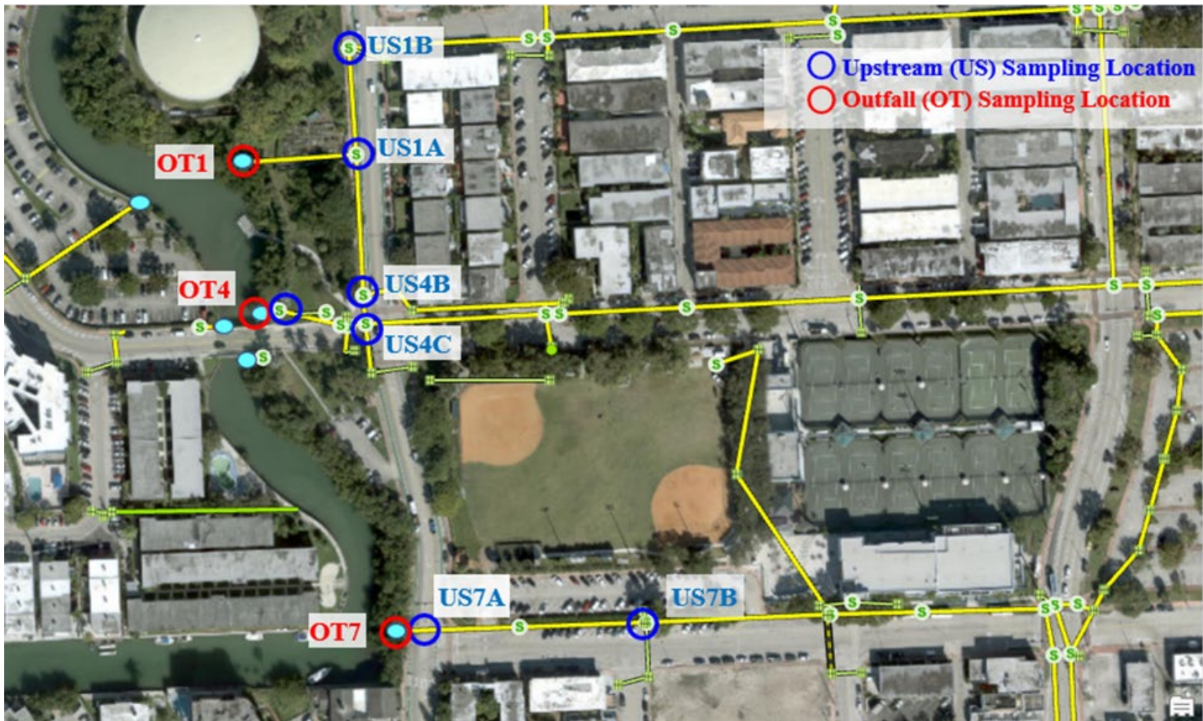
Figure II.5: Sampling locations of the upstream (US) and outfall (OT) shown in the blue and red circles within the map. Original map provided by the CMB containing data collected by E Sciences Inc.
