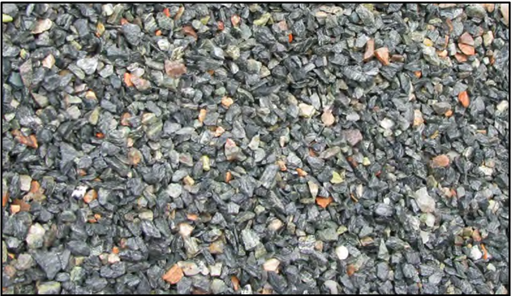
G-1 GRAVEL WALKWAYS: 3/8IN Ø CRUSHED GRANITE
