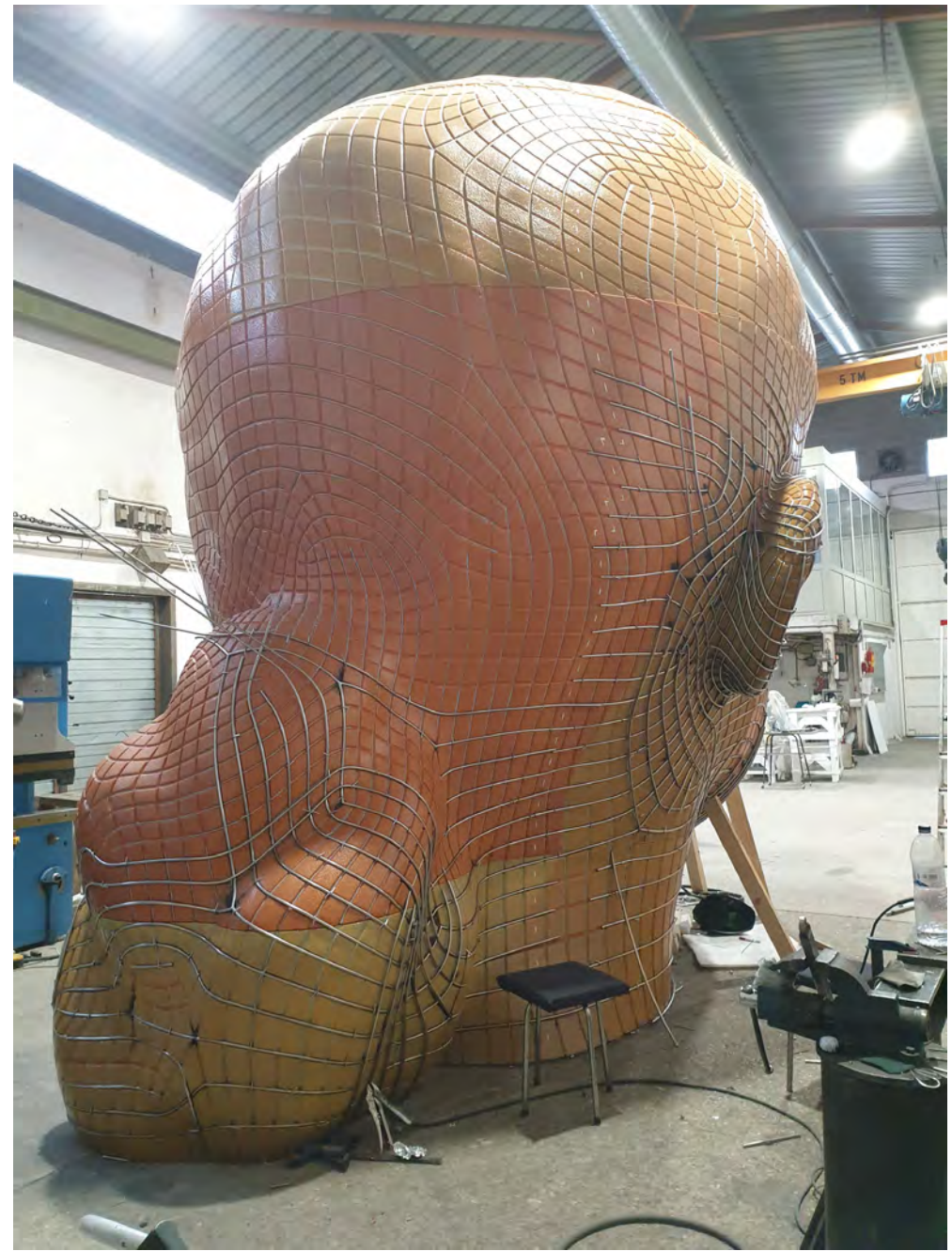
Images from the fabrication process of Minna , on the polystyrene mold.
