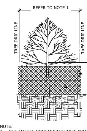
1. DUE TO SITE CONSTRAINTS TREE PROTECTION FENCE MAY BE CONTINUOUS TO PROTECT MULTIPLE TREES. TREE PROTECTION FENCE TO BE INSTALLED AT EDGE OF EXISTING HARDSCAPE. WHERE SPACE ALLOWS TREE PROTECTION FENCE TO ALIGN WITH
